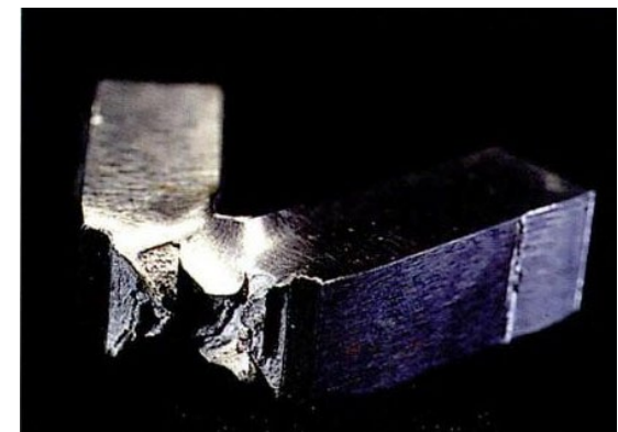
Modern high quality steel - Ductile fracture
