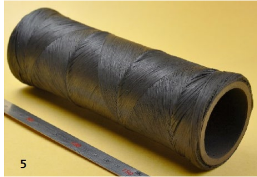
Curved tile made of SiC/SiC SiC pipe reinforced with SiC/SiC SEM image of microstructure
